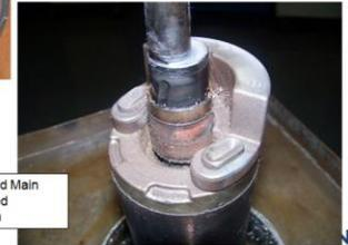
Seizure Of The Relatively Lightly Loaded Main Bearing And Low Amounts Of Recovered Oil Are Evidence Of Loss Of Lubrication
