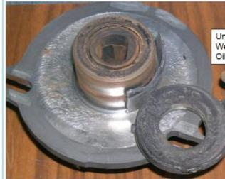
Unloader Bushing Seized To Drive Bearing, Excessive Wear On Thrust Surfaces And Low Amounts Of Recovered Oil Are Evidence Of Loss Of Lubrication
